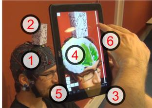
**Figure 2. Mind-Window system overview.** (1) EEG cap, (2) 3D AR marker, (3) tablet PC, (4) virtual brain representation, GUI: button bar (5), slider (6)
