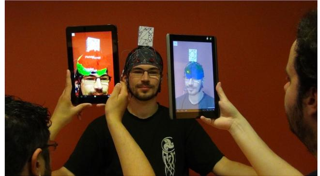
Figure 1. Our novel “Mind-Window” approach enables one or multiple users to visualize in situ the brain activity of a person in real-time by using tablets and augmented reality. The display of the virtual brain is updated in real-time according to the real brain activity of the person which is measured thanks to an electroencephalography (EEG) cap.
